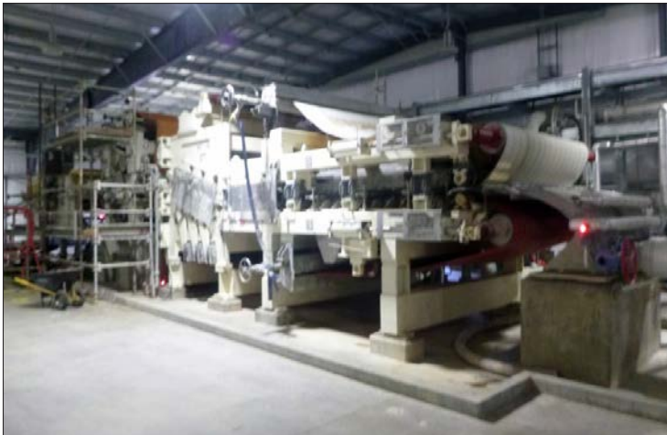
Hymac Wetlap Machine Model 100 HP-SF with Heavy Duty Press Reconditioned 2018 (Rated 400 ODSTPD)
